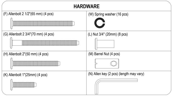
Do not fully tighten all bolts until all parts are in place. (please add an extra 1/2 revolution to the bolts when using spring washer after tightening)
